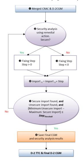
If the level is secure or can be made secure by optimizing remedial actions, the coordinated capacity calculator will then test a higher value of TTC. Otherwise, it will then test a TTC value in between the
