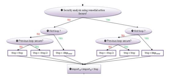
The dichotomy is set with a 50 MW step in order to optimize the capacity offered to the market while reducing the computation time. Considering optimal remedial actions have been applied in each step of CC, the dichotomy approach guaranties final solution is less than 50 MW suboptimal compared to absolute maximum Italian import.
