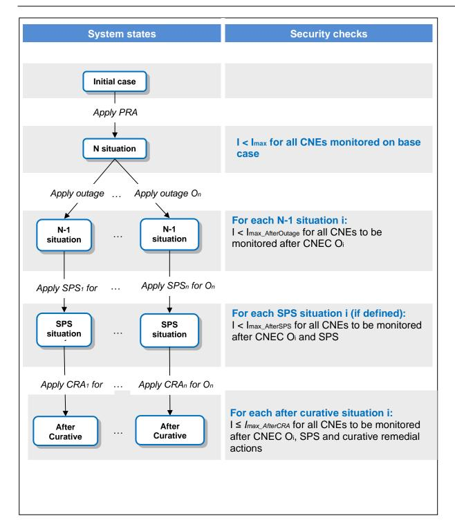
In order to prevent overloading of network elements that are influenced by the application of cross-border-impacting remedial actions during the CC in export direction from Italy, these network elements can be included as MNEs in the RAO. For each MNE i in a contingency case, the following has to hold:
