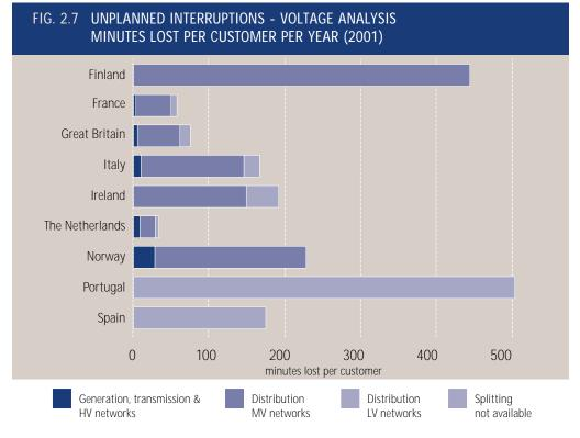
Voltage Level Analysis -Unplanned Interruptions (2001 National Data) Figures 2.7 and 2.8 show unplanned interruptions in 2001 split into three main categories (Generation, Transmission and HV network (> 35kV); MV network (1kV-35kV) and LV network) according to voltage level.
